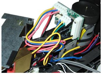
Installation section. A detail is shown to the right of the "Cruise On/Off" switch connection. Note the connection on the far left 2 pins, and verify you can see 4 unconnected pins to the right of the plug, indicating that indeed the left 2 pins are connected to the plug. **Damage will occur if done incorrectly**.
