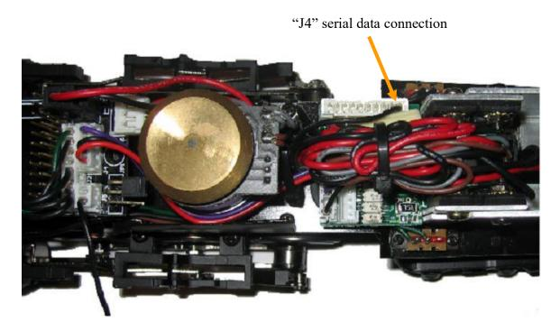
4) Locate the serial data line cluster wire nut, and attach the wire from "J4", pin-1 to this cluster and replace the wire nut.
