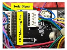
The picture to the left shows this board and the location of the serial output. In this picture the pin with the two purple wires connects to the sound board and to the
