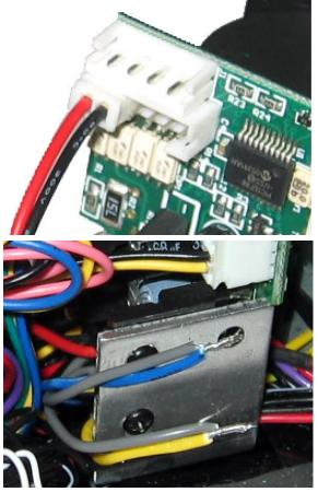
When using the temporary splices, place a piece of heat shrink (do not shrink), to protect the wires from shorting to the frame or to each other. Shown above is the temporary wiring prior to testing the engine.
