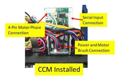
Mount the new CCM using the old heat sink and in the same location as the old unit. Next attach the original cables to the CCM as shown.
