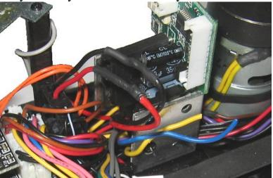
There will be a 6-pin Molex connector that supplies power and motor connections (hidden and located at the base of the command board). Cut the 4 wires going to the connector. These wires are usually Red (3<sup>rd</sup> rail), Black (common), Blue and Yellow (motor brushes). These wires will need to be spliced into the 4-pin Black Molex connector provided that attaches to the CCM.
