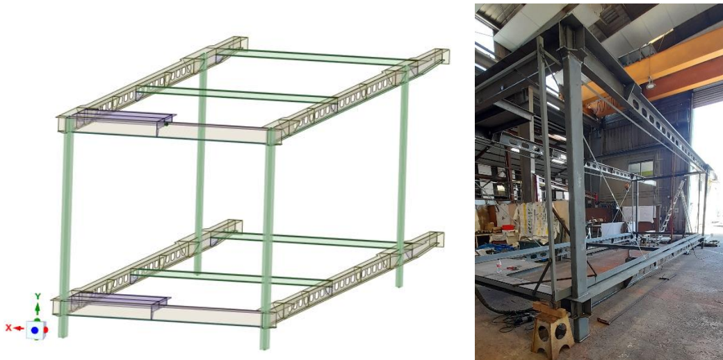
Figure 2.5. Structure of cabin model “Ramsess”
