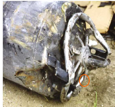
PRD location was plugged using a threaded cap
