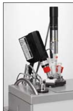
Dip-pipe installation is used for monitoring in a production scale crystallizer.
