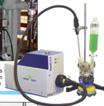
Multiple reactor systems provide the ability to perform parallel experiments to efficiently map the crystallization operating space.
