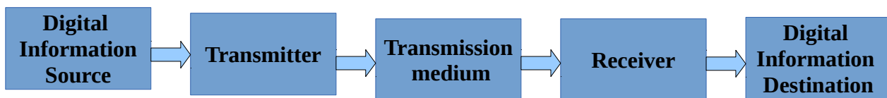
Fig.2. Simplified Block Diagram of a two-station data communications circuit.
