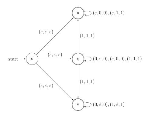
When verifying that x \* y = z, t is the node which is used as long as x and y are both not exhausted; u is the node to be used when the end of x is reached while the end of y has still to be found while v is the node to be used when the end of y has been reached while the end of x has still to be found. There are transitions on empty tuples from s to all of these three nodes as the two extreme cases that one of x and y is  $\varepsilon$  need to be covered as well.
