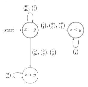
Here  $\binom{a}{b}$  on an arrow means that the automaton always goes this way.
