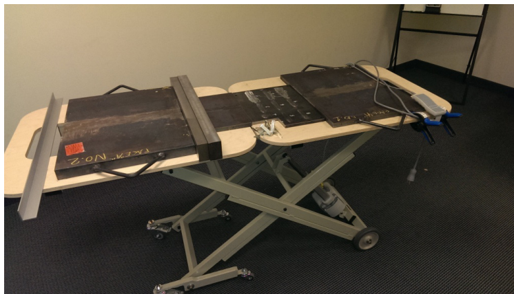
Figure 11 Test plates and calibration test blocks with an electric height adjustable mobile table for ergonomcy
