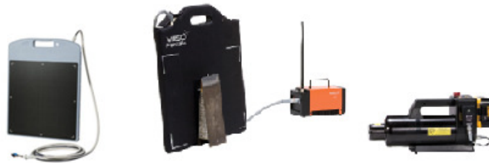
Figure 2 DR system showing a wireless module and a portable X-ray tube - courtesy GE & Mistras/VMI
