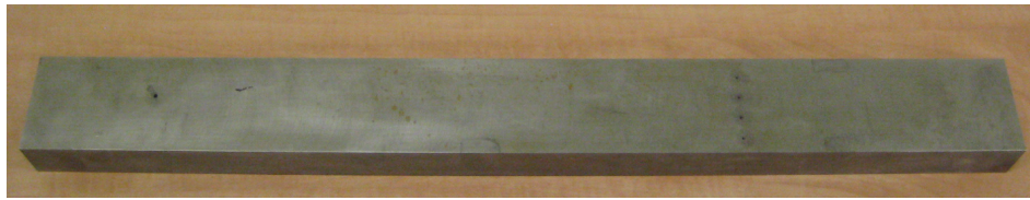
Figure 12 Calibration block in CSA 300W material 700mm long by 38mm thick by 70mm high, four ( 4 ) - 1.5mm SHD & one ( 1 ) - 3mm SHD, use a straight edge along the length for probe stability while performing TCG calibration
