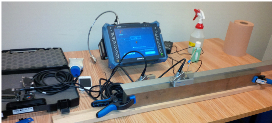
Figure 14 Set-up for TCG Calibration of the 16 element 5 MHz probe Olympus 5L60 A14
