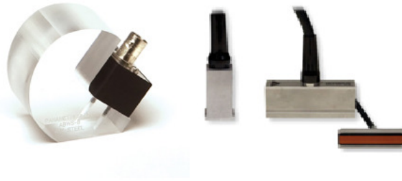
Figure 4 Conventional UT AWS Snail wedge probe & Phased Array probe courtesy Olympus
