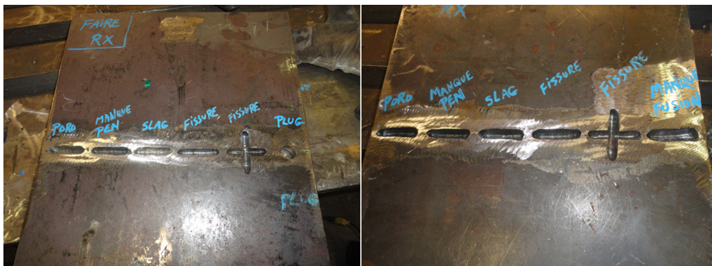
Figure 9 : 300W test plates 24" x 18" & 0.75" and 1.5" thick from left to right, with gouged cavities to introduce real defects, porosity, lack of fusion, slag, crack, crack and crater crack in a plug weld or lack of fusion respectively.
