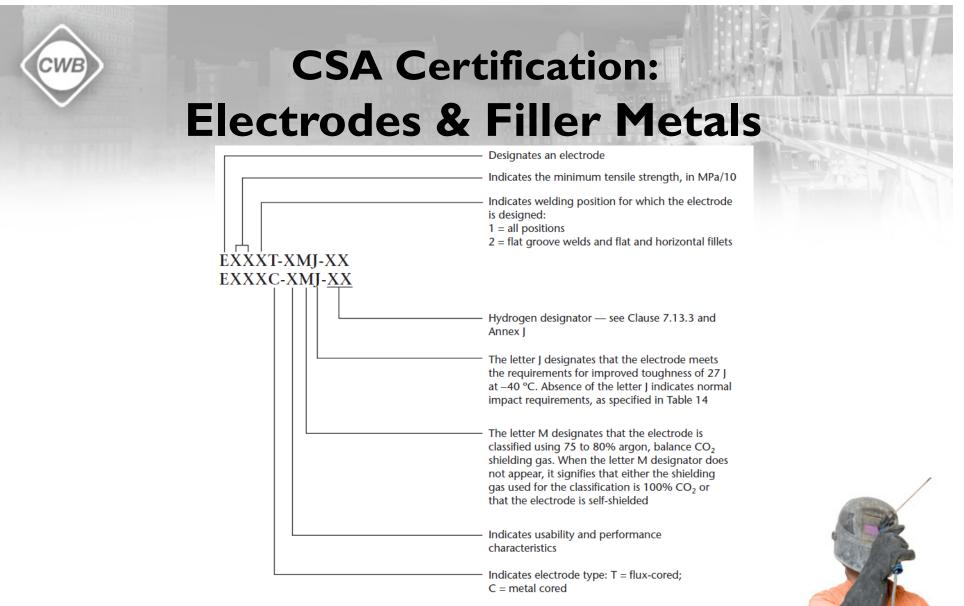
Figure C.1 Method of classification for carbon steel electrodes for flux- and metal-cored arc welding
