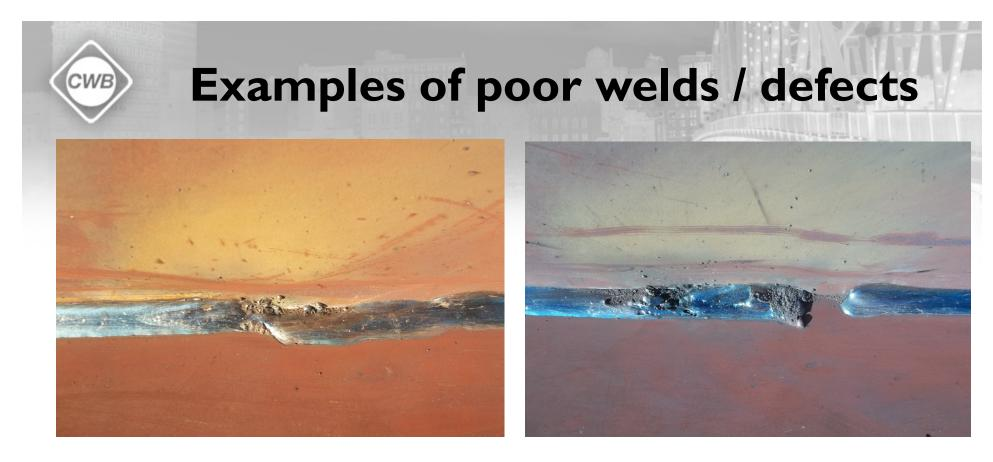
Incorrect profile and out of line weld
