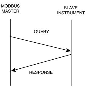
Figure 1. Modbus Link Layer
