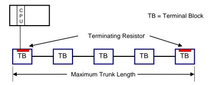
The maximum trunk length can be doubled by using a "T" topology as show below. Note the location of the terminating resistors.
