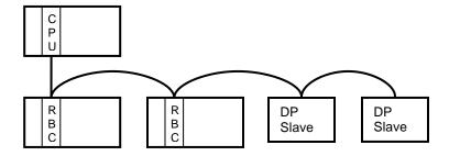
Up to 32 devices can be connected on a single segment. To increase distance or the number of devices supported, segments can be interconnected by using repeaters. Up to 10 segments may be connected together.
