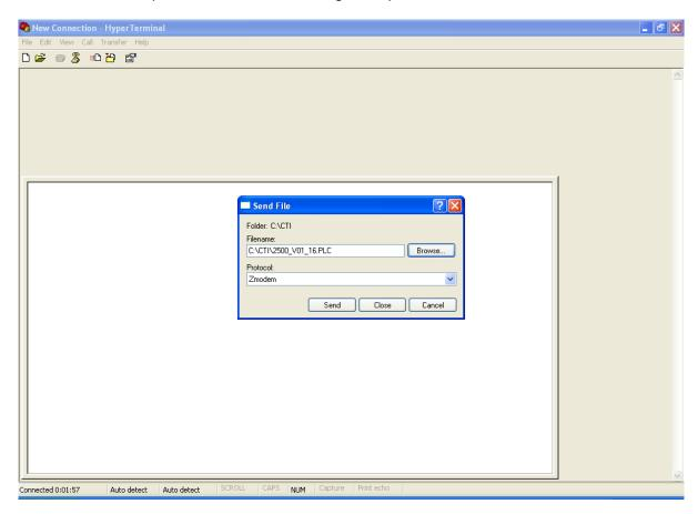
8. Start the file download by pressing 'Send'. HyperTerminal displays a window showing the status of the file transfer. Once the transfer is initiated, the MSD should should display "U02"
