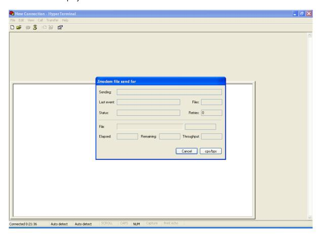
Once the transfer has completed successfully, the MSD should display "U06", indicating the controller is starting to write the new firmware to flash memory. The decimal points will flash in sequence to indicate progress.
