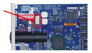
The user jumpers are located next to the user switches (labeled as
