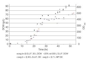
Figure 2. Plot of dry cell weight (DCW) and culture density for exponential-fed batch *P. pastoris* batch cultures from the 7 L SIP, and S.U.F. fermentors. The switch from glycerol feed to methanol feed is apparent at around 28 hours with the notable growth rate change. The final OD<sub>600</sub> of these cultures reached about 600.
