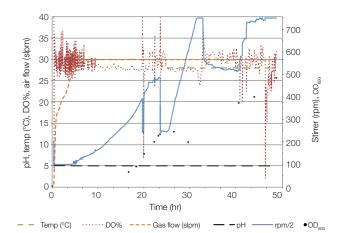
Figure 6. Graph of a routine 7 L glycerol- and then methanol-fed *P. pastoris* culture in a Sartorius 10 L stainless steel SIP fermentor. Air at 30 slpm was used starting at about 4:30 hours. Starting at around 34 hours,  $O_2$  was supplemented to maintain the DO at a set point and reached 100% by 47 hours.
