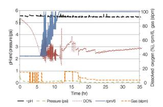
Figure 8. Glucose-fed 30 L *P. pastoris* batch culture. Oxygen was supplemented up to 1 slpm.
