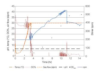
Figure 11. Comparative 7 L *B. subtilis* culture grown in the 10 L stainless steel Sartorius SIP fermentor.
