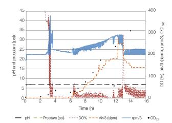
Figure 10. A *B. subtilis* culture growth in the 300 L S.U.F. at 20% working volume (60 L). Yields were comparable to those of typical cultures in a 10 L stainless steel SIP fermentor.
