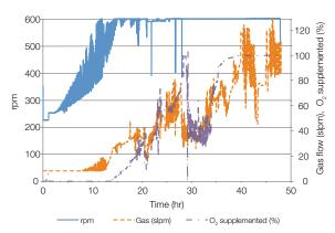
Figure 4. Graph of average (n = 3) agitation, total gas flow, and oxygen supplementation for three exponential-fed *P. pastoris* bath cultures in the 30 L S.U.F. Peak gas flow reached 5 vvm. The reduction in gas flow at around 28 hours is due to induction with the change from glycerol to methanol as the feed substrate. Flow rates were comparable to those performed in Sartorius 10 L stainless steel fermentor.
