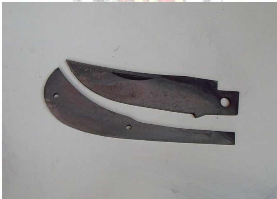
Blade and spring right after air quench.
