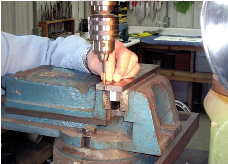
Cleaning scale from pivot hole in blade using an expandable brass reamer and grinding compound.
