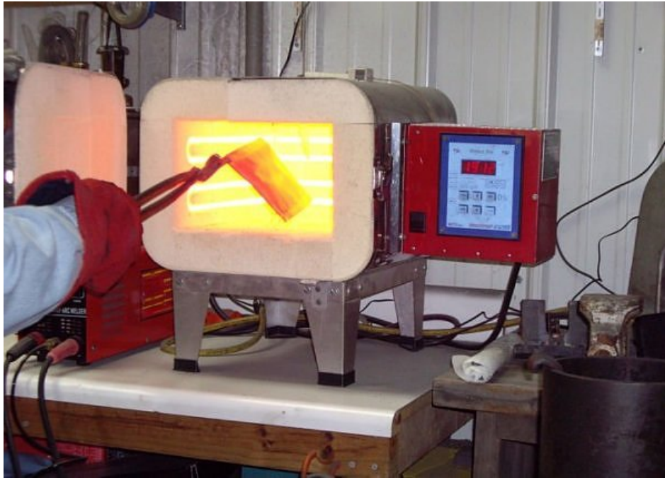
Blade and spring coming out of kiln to air quench.
