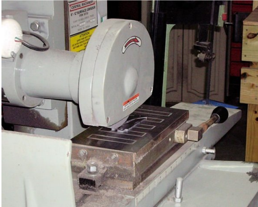
Surface grinding heat-treat scale from blade and spring.
