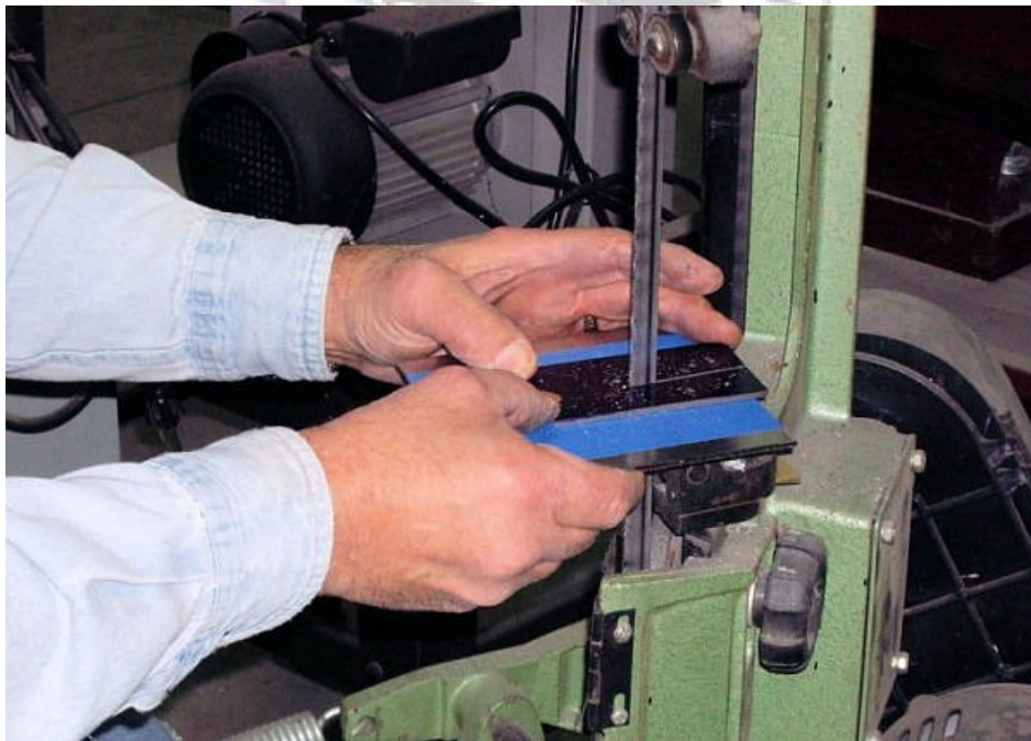
Sawing out the blade and spring.
