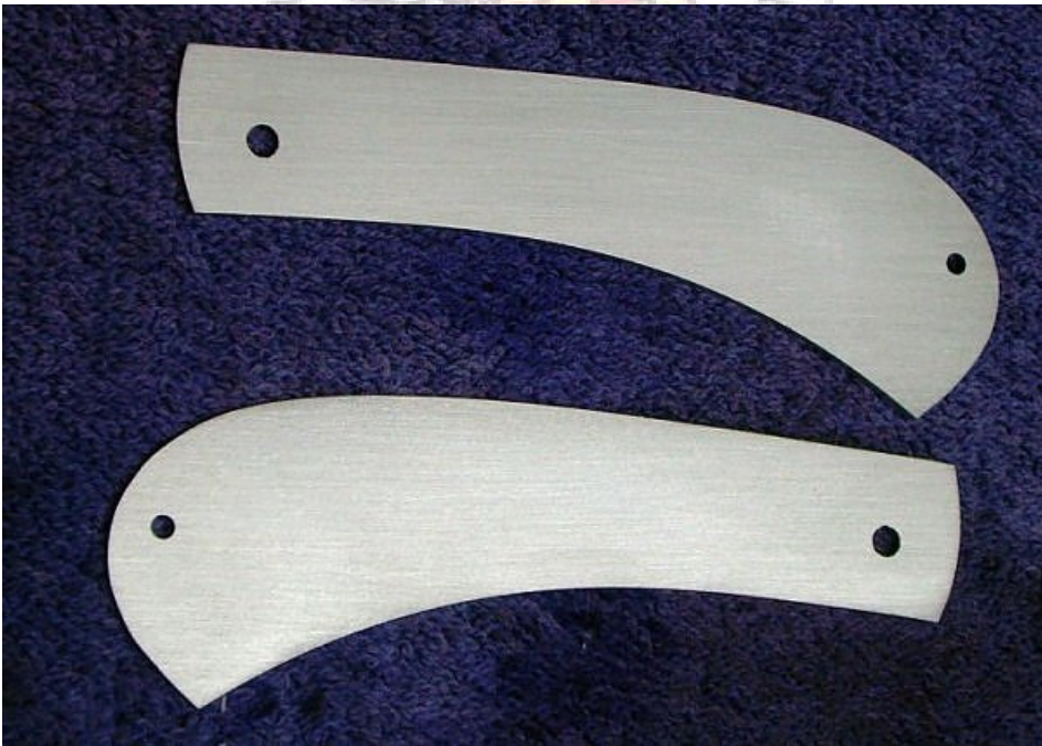
Liners flat, clean and ready to weld bolsters on.
