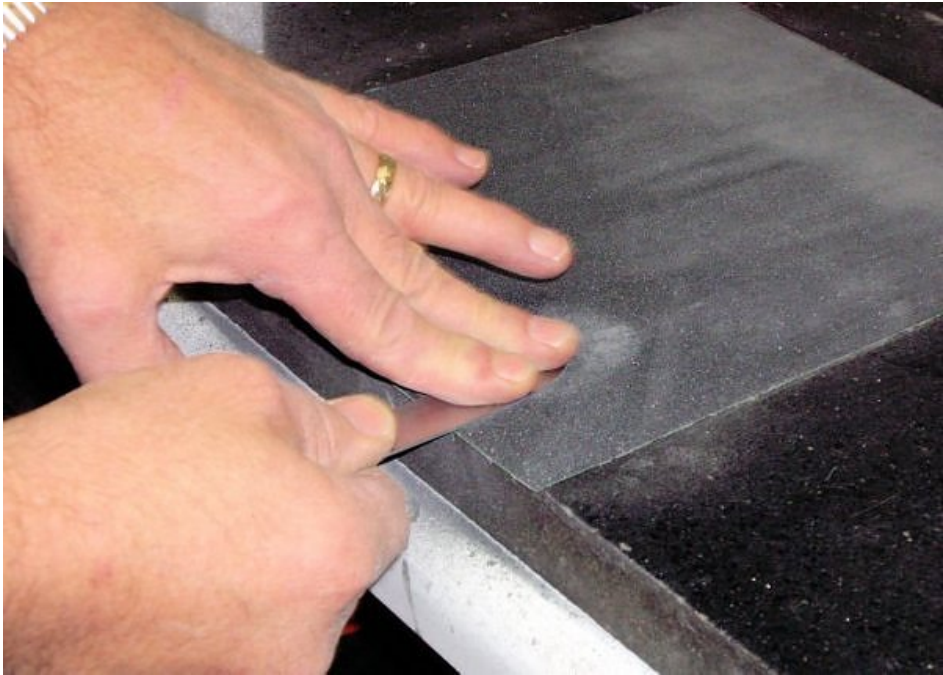
Liners flat, clean and ready to weld bolsters on.
