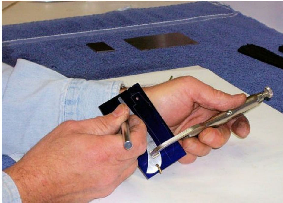
Sawing out the blade and spring.
