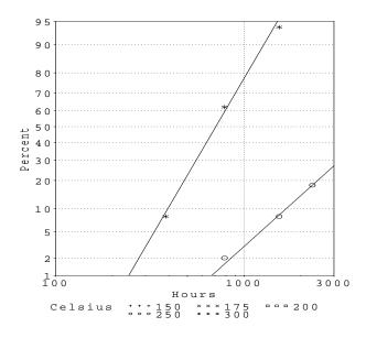
Figure 4: Lognormal probability plot of the failures at 250 and 300°C for the new-technology integrated circuit device ALT experiment.
