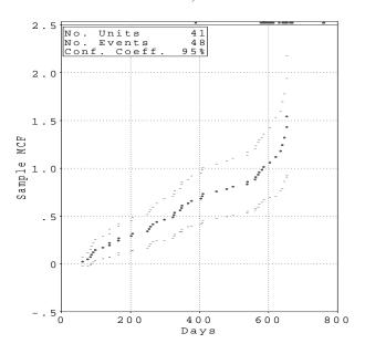
Figure 7: Estimate of the mean cumulative number of valve seat repairs.
