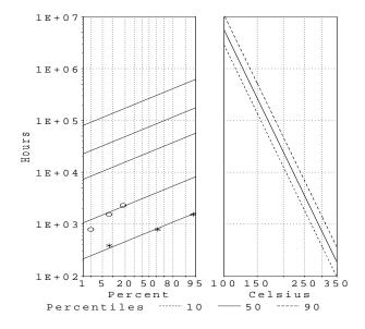
Figure 5: Lognormal probability plot showing the Arrhenius-lognormal model ML estimation results for the new-technology IC device.
