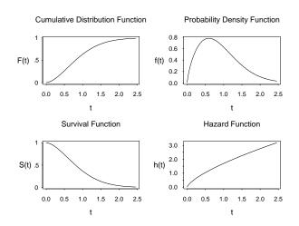
Figure 1: Typical time-to-failure cdf, pdf, sf, and hf.
