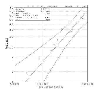
Figure 2: Weibull probability plot with the Weibull ML estimate and a set of approximate 95% confidence intervals for F(t) for the chain link failure data.
