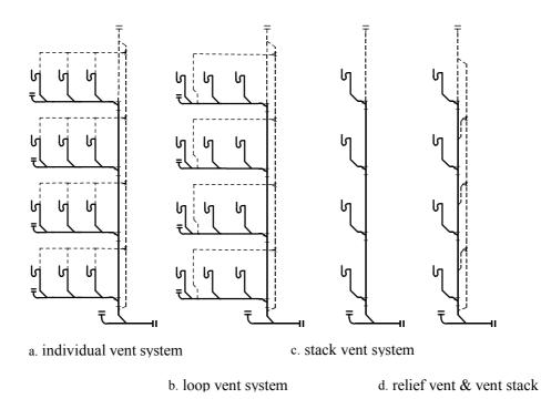
Figure 6. Types of the vent pipe for building drainage system
