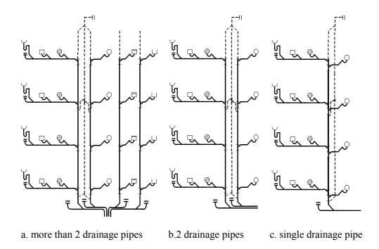
Figure 5. Types of building drainage pipe for building drainage system
