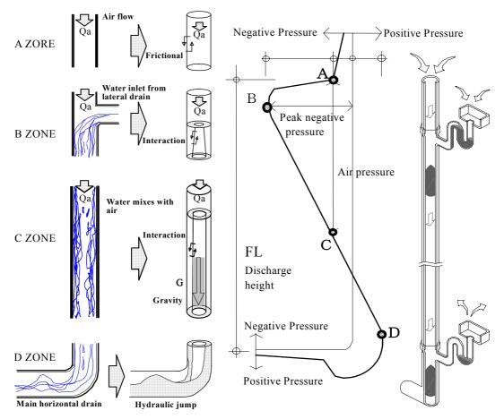
Fig.1 Mechanism of vertical drainage feature and inverted model
