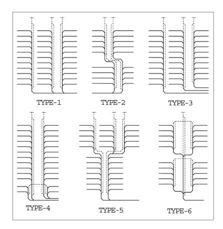
Figure 12 Drainage construction categories for current high-rise buildings
