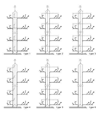
Figure 9 Categories of partial detail drainage loop vent construction
