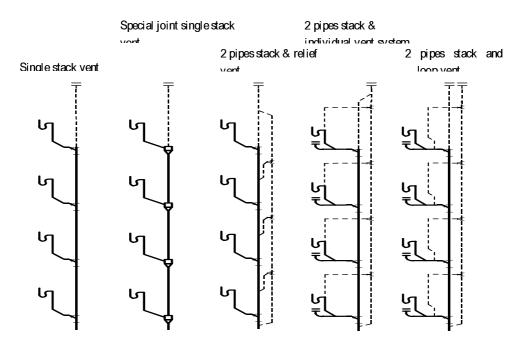
a. Single-pipe drainage & vent system b. Two-pipe drainage & vent system
