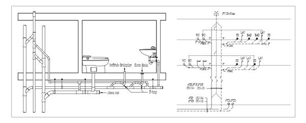
Figure 10 a typical partial detail of drainage plumbing construction
