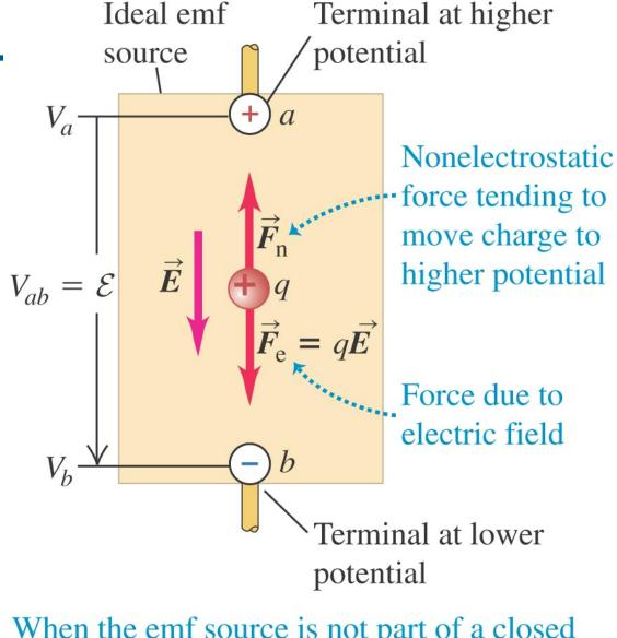
When the emf source is not part of a closed circuit,  $F_n = F_e$  and there is no net motion of charge between the terminals.
