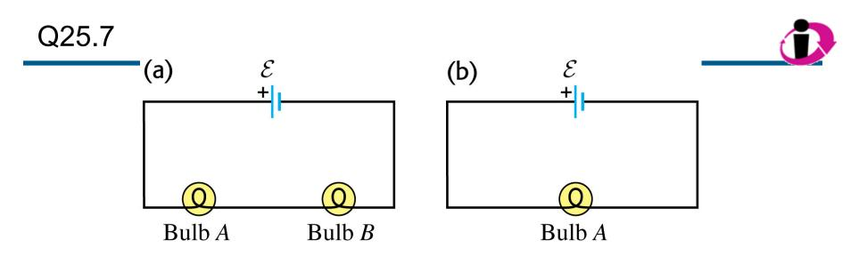
In the circuit shown in (a), the two bulbs *A* and *B* are identical. Bulb *B* is removed and the circuit is completed as shown in (b). Compared to the brightness of bulb *A* in (a), bulb *A* in (b) is
