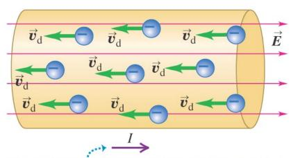
In a metallic conductor, the moving charges are electrons — but the *current* still points in the direction positive charges would flow.
