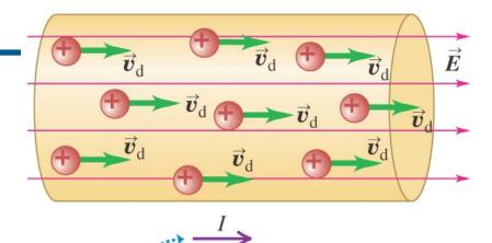
A **conventional current** is treated as a flow of positive charges, regardless of whether the free charges in the conductor are positive, negative, or both.
