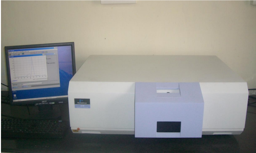
Photoluminescence spectrophotometer for studying Luminescence properties liquids, solids and films
