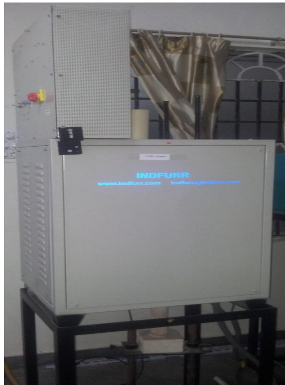
Vertical Bridgmann set up for single Crystal growth – Temp 1400°C
