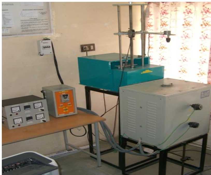
Czochralski set up for metallic single crystal growth – Temp 1400°C
