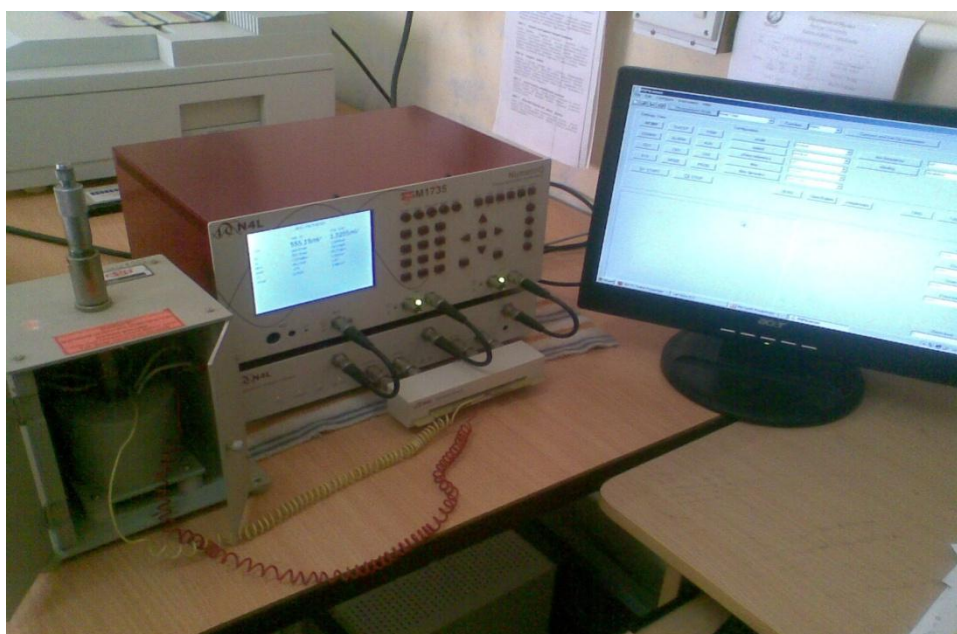
Phase Sensitive Multimeter interfaced with Impedance analyzer for studying the electrical properties solids and films (RT to 400°C)
