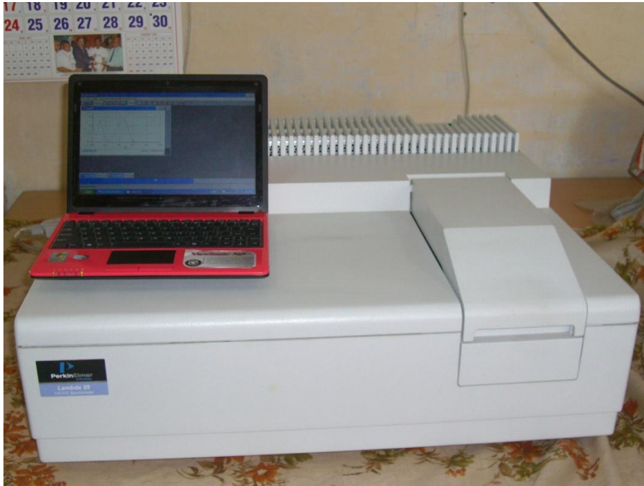
UV-VIS-NIR spectrophotometer for studying the optical and electronic properties liquids, solids and films
