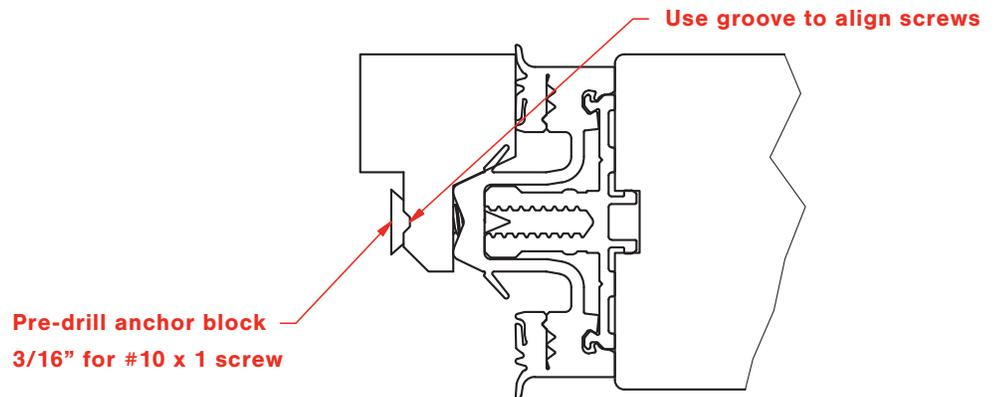
4. **Install and set the door unit plumb, level, and square into the rough opening. Ensure that framing shims have been placed between the jamb and the stud directly behind hinge locations.**
