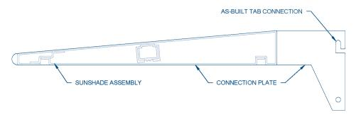
Figure 8 – Geometry of sunshade connection plate as observed in field. Shop drawings indicated top-bolted connection was intended to be a standard hole, not a tab.
