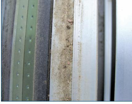
Figure 4 – Dust/ debris within disassembled snap connection.
