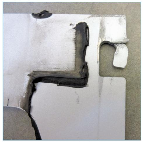
Figure 10 - Failed tab connection at top bolt hole of sunshade connection plate.
