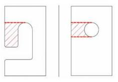
Figure 11 – Shear planes for tab and standard hole-connection details.
