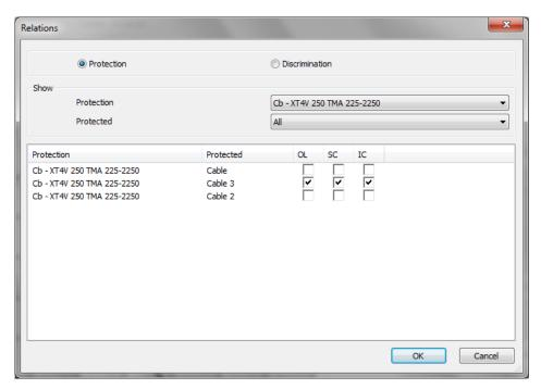
**Discrimination:** creates a discrimination link between two circuit breakers. Verifications are made according to QT1. The dialog window shows the following values:
