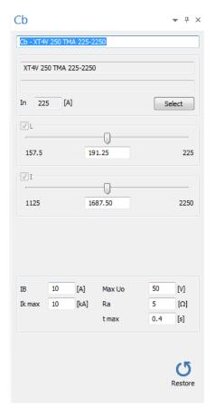
Changing the breaker I<sub>B</sub> (the load current of the breaker), it is possible to appreciate the curve variation due to it.
