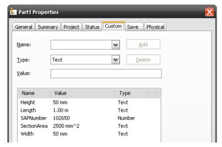
After a few changes the Custom tab of iProperties looks a little different, but there is no visual change to the Parameters box. It appears that this could all be done through the iProperties box naturally, but in this manner the user can create equations with their parameters and easily linked the dimensions from their sketches to the appropriate downstream items.
