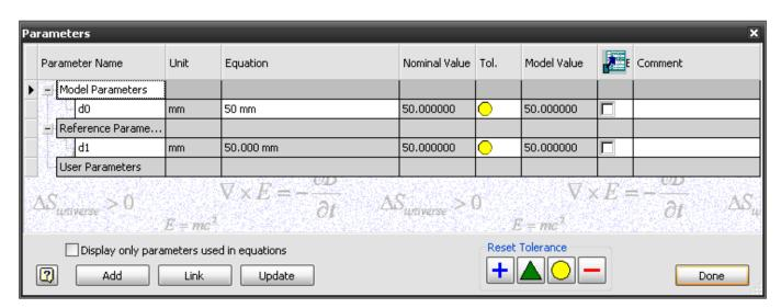
Inside the Parameters box you can create your own Parameters as well known as User Parameters by using the Add button. Existing Model and Reference Parameters can also be renamed for clarity.
