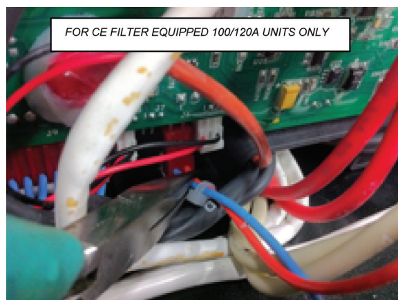
Figure 13: CE Filter Units ONLY. Remove and replace 'J6' Connection
