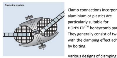
Clamp connections incorporating aluminium or plastics are particularly suitable for HONYLITE<sup>™</sup> honeycomb panel. They generally consist of two parts with the clamping effect achieved by bolting.
