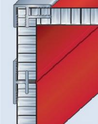
For fascia cladding applications special aluminium sections are provided for clamp connections.
