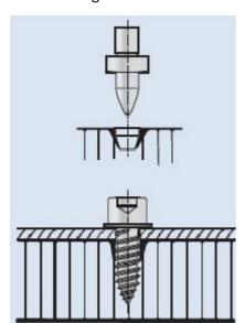
In the case of threaded fasteners higher pull-out strength can be obtained due to the larger contact area of the screws.
