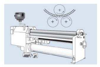
The surface should be protected from damage by affixing plastic strips of 1mm to 2mm thickness during processing.
