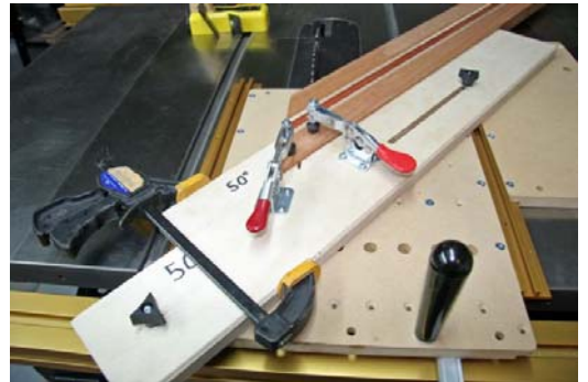
12. The hold-down clamps and handle that has been added to the sled make this a very safe process.
