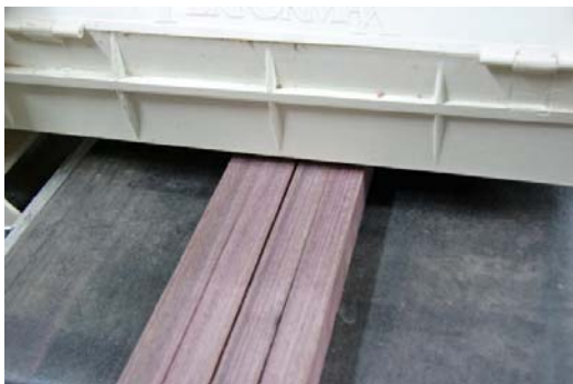
8. Sand common strips on edge for consistent thicknesses.
