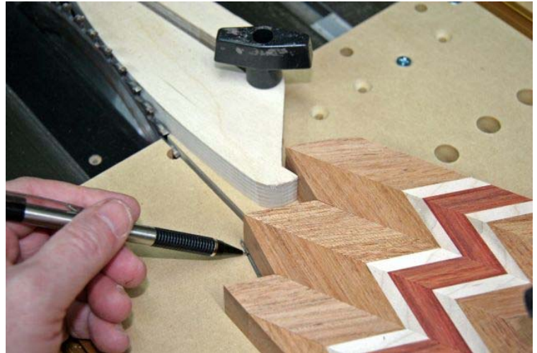
22. When the last ear is at the registration point, draw a profile of an ear for manual positioning.
