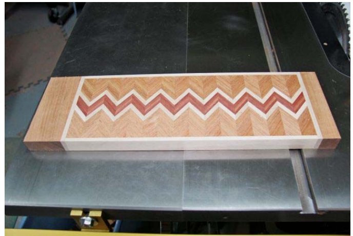
29. Once flush, add the Maple border to the short edges along with the Jatoba ends. Finally, add the Jatoba to the long edges (not shown).
