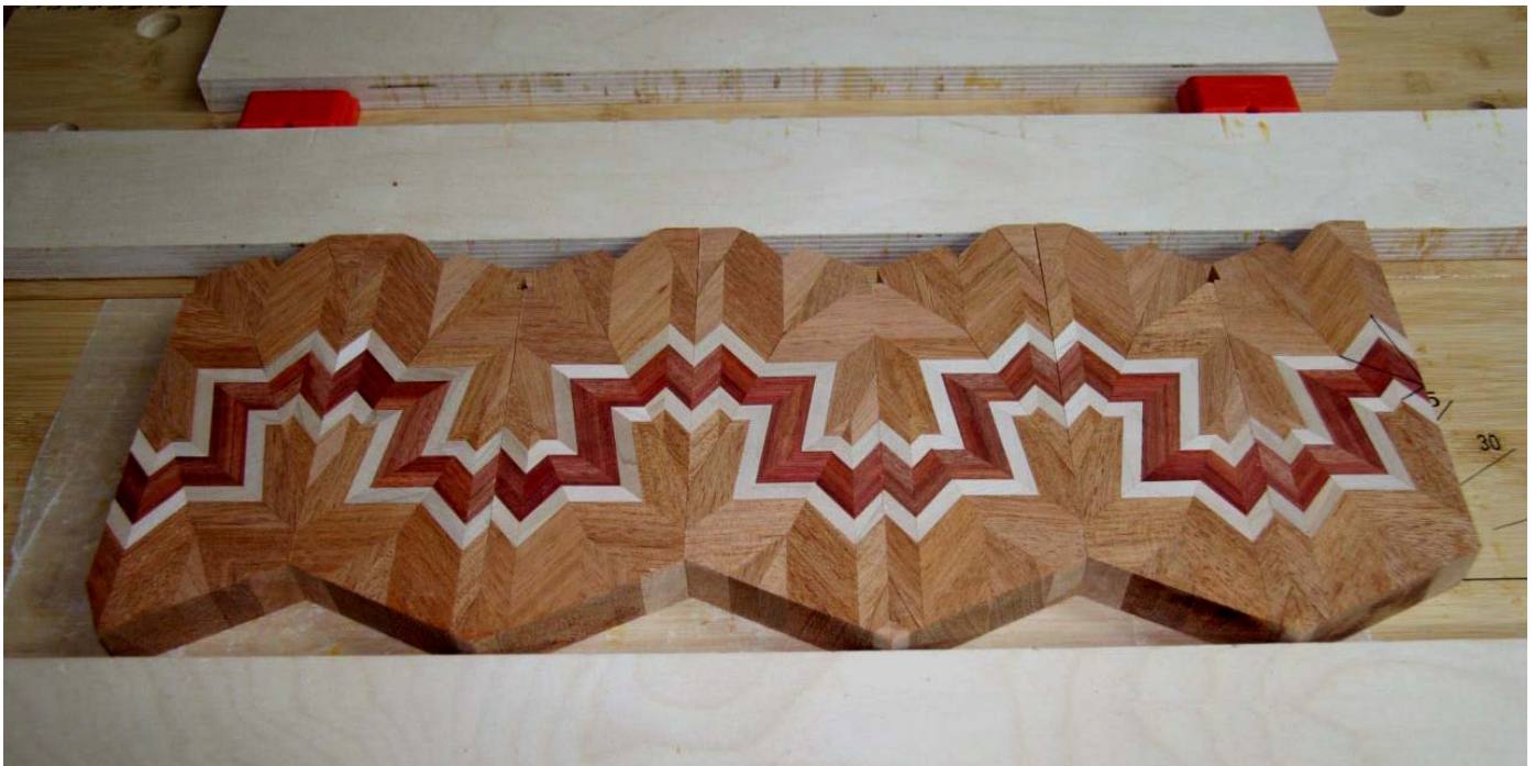
27. The completed 3rd generation board in the clamping channel. The channel has done its job nicely as the pattern is nearly perfect.
