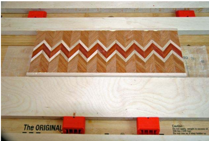
28. You can use the clamping channel to add the Maple border to the long edges.
