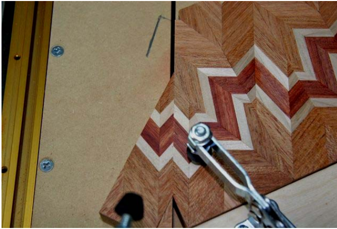
25. The pattern is not symmetric so an adjustment to the stop is needed. 26. The board is now ready to cut into strips for the 3rd generation.
