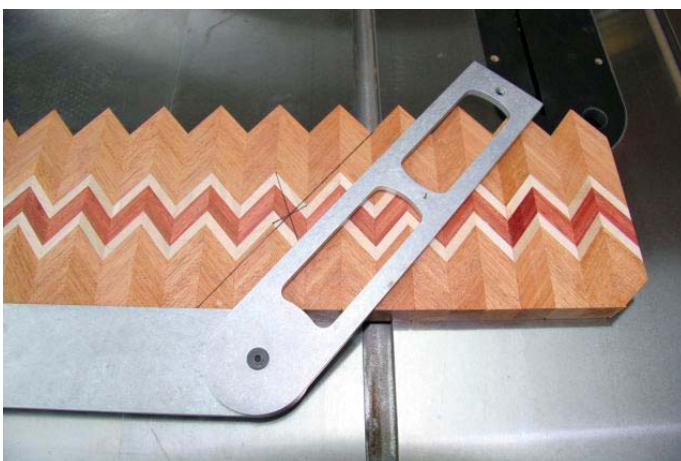
17. Use an angle protractor to draw a line indicating where the next cut will be made. This line will help in the positioning of the board.
