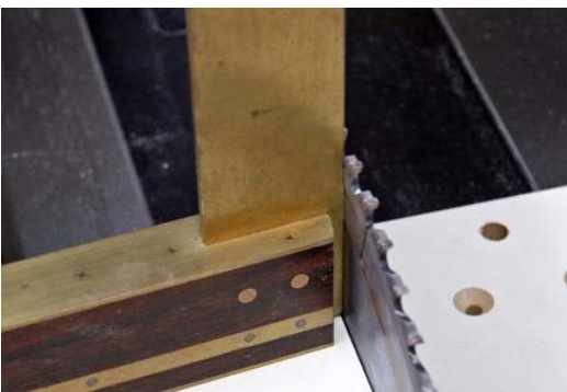
10. The saw blade must be exactly 90° to the table if the laminated pattern is to be accurate.
