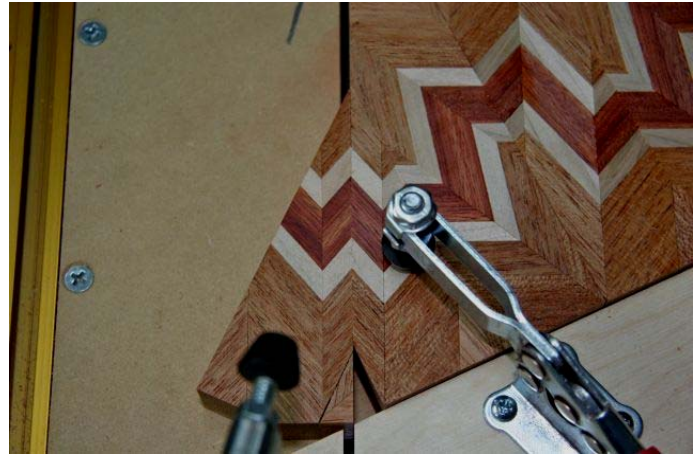
25. The pattern is not symmetric so an adjustment to the stop is needed. 26. The board is now ready to cut into strips for the 3rd generation.
