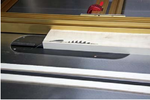
7. The INCRA TS-LS Table Saw Fence is the safest and most accurate way of cutting thin strips.
