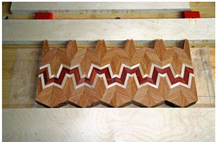
23. Assemble the strips, flipping alternates edge-for-edge and use the clamping channel to slide the strips into position before gluing.
