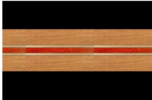
1. All three boards will start with the same 1" thick laminated board cut into 7/8" wide strips at 50°.
