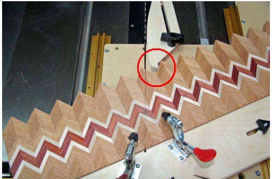
19. Move the registration block so that it is in firm contact with the ear that is closest to the blade. This provides the point of registration which will be used to reposition the board for repeatable cuts.
