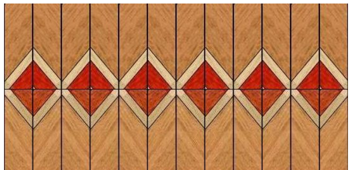
30. Cutting a 1st generation chevron pattern and then sliding the top over the bottom always yields a diamond pattern.
