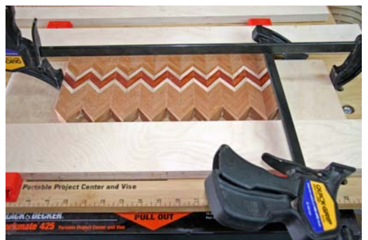
14. Tighten the clamps, alternating between the channel vise and the horizontal clamp.
