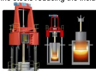
ESR: (Electro-Slag Remelting) to refine steels reducing the inclusions
