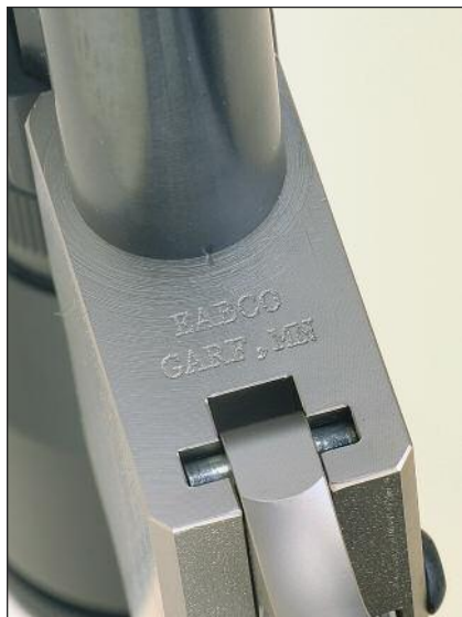
All machining is top rate, as witnessed by the detail shown here where the barrel meets the receiver.
