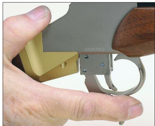
To close the action, finger pressure is used to lift the falling block into place.
