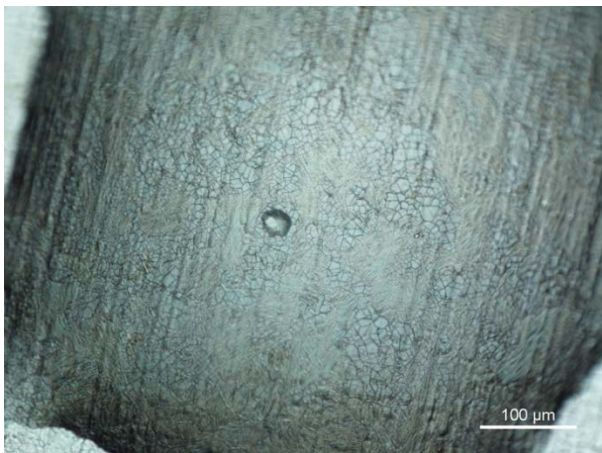
Figure 10. 20x optical microscope ( 620 \times 620 ) \mu\text{m}^2 image of 100 nm MLGr/Ni. A bubble is formed on the surface, after depositing 0.5 M \text{H}_2\text{SO}_4 droplet and waiting overnight.
