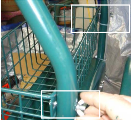
Once both bolts are in, tighten the wing-nuts
