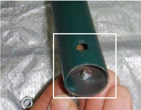
Removing bolts at the end of the cart handle
