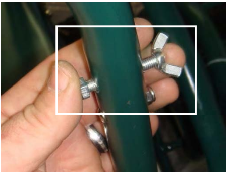
Remove the bolts with the wing-nuts from the cart frame handle
