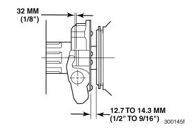
Figure 14 — Verify Clutch Release Yoke Free Travel and Release Bearing Travel
