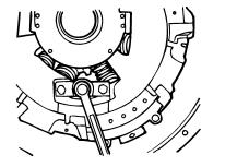
Figure 8 — Box Wrench Installed on Kwik-Adjust™ Component
