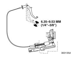
Figure 5 — Verify Clutch Brake Squeeze
