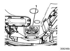
Figure 10 — Clutch Adjustment Lock Plate
