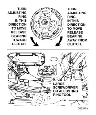
Figure 11 — Adjusting Clutch
