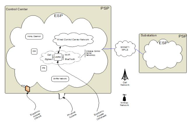
Figure 2. Typical electronic security perimeter (ESP) for a utility
