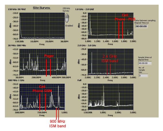
Figure A-2. Frequency sweep of 150KHz – 3GHz
