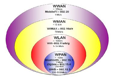
Figure A-1. Wireless standards and associated technologies
