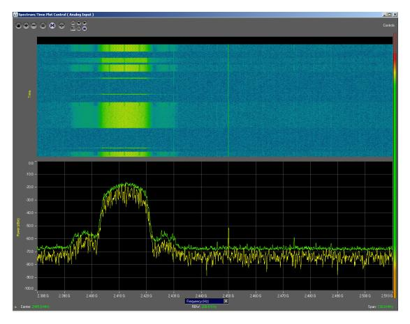
Figure A-3. Time-frequency sweep of 802.11b network
