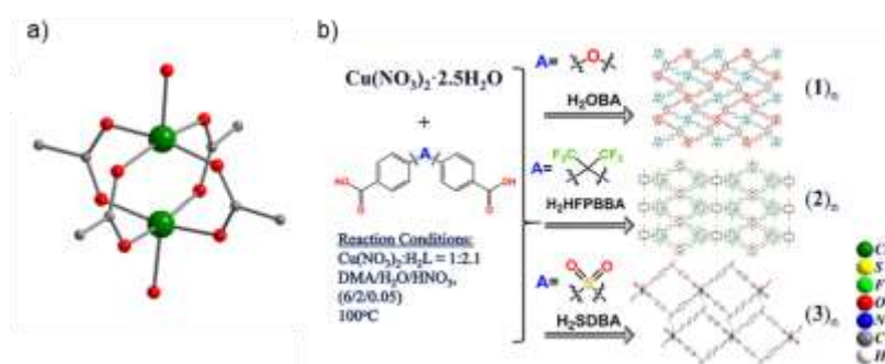
Figure 1: Representation of a) the dinuclear [Cu 2 (COO) 4 (DMA) 2 ] paddle-wheel SBU and b) the general synthetic scheme employed for the synthesis of compounds ( 1 ) n - ( 3 ) n discussed in this study.
