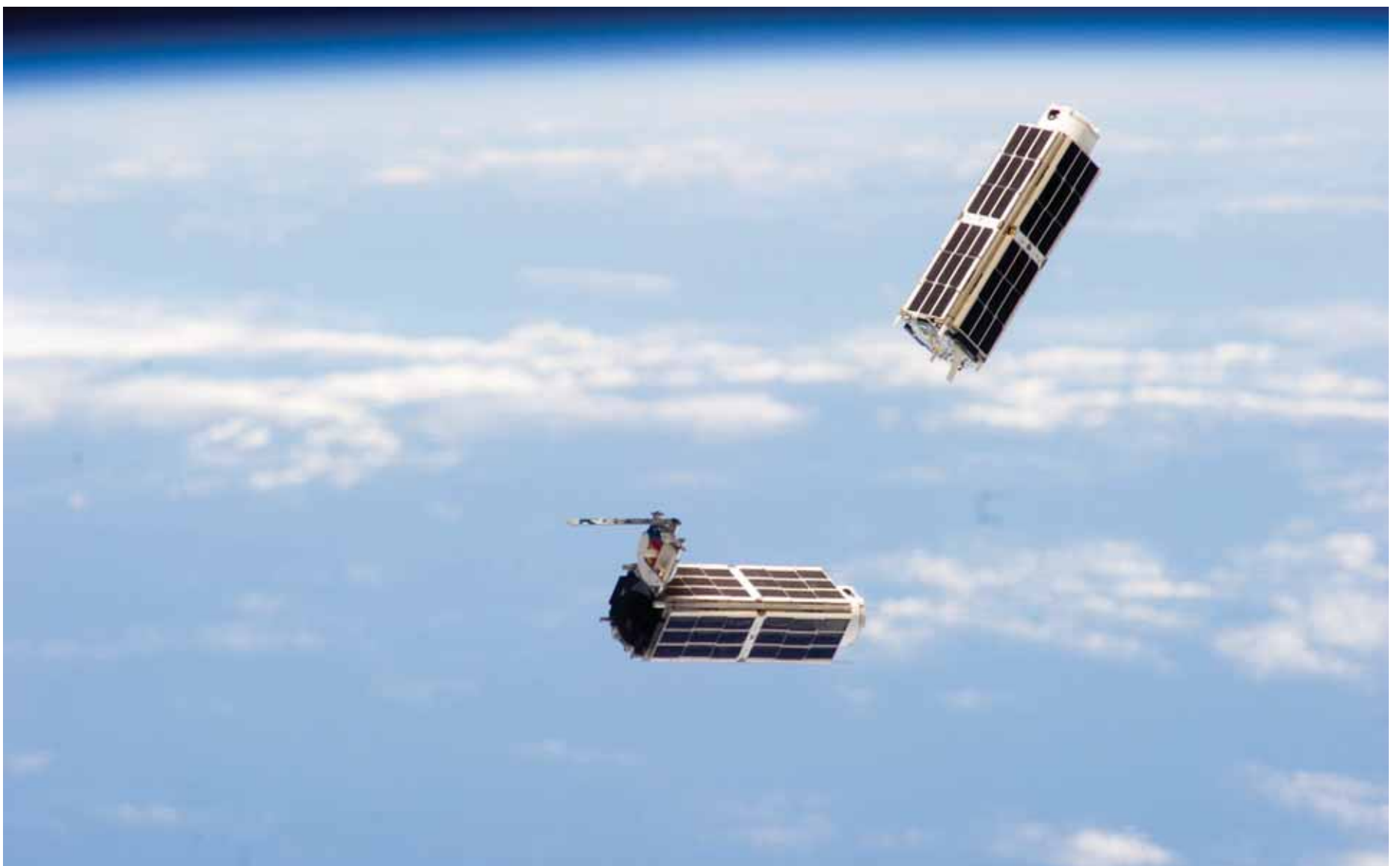
SLICK: A set of NanoRacks CubeSats is photographed by an Expedition 38 crew member after the deployment by the Small Satellite Orbital Deployer (SSOD). The CubeSats programme contains a variety of experiments such as Earth observations and advanced electronics testing.
