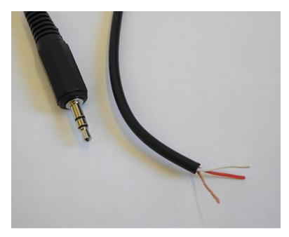
(3) Strip off approx. 1/16in of the insulation of the white and the red wire, twist the exposed ends of the white and red wire together and cover with solder, also cover the copper wire with solder – do this for both cable ends:
