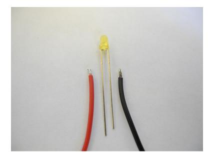
Solder the red wire to the LED's long leg and the black wire to the LED's short leg, cut the legs first, to have only very little unexposed conductors:
