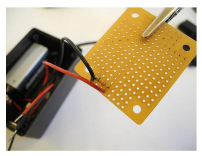
Use the circuit from page 7 to see how parts connect on the printed circuit board. Try and build everything on one side of the circuit board, so that the circuit fits next to the 9V battery in the project box. Also, as a building tip: use the legs of components on the underside of the printed circuit board to make connections like this:
