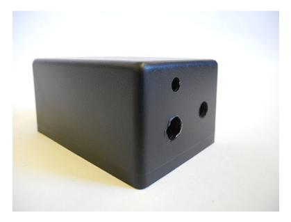
The holes for the components were drilled with the following bits:  $\frac{1}{4}$ " for the toggle switch,  $\frac{5}{16}$ " for the audio jack and  $\frac{11}{64}$ " for the audio cable out (on the opposite side of the box, see below).
