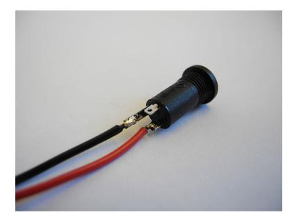
It is a good idea to "thin out" the ends of the wires that are not soldered to the jack before tinning them. Just separate 3-5 strands of the exposed end and cut them off before testing the rest of the strands together and covering them with solder. This way they will fit better through the PCB holes.
