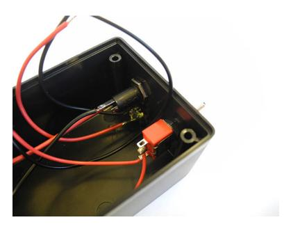
On the other side of the box insert the 12 inch long audio cable. Tie a knot into the cable as a strain relief on the inside of the box:
