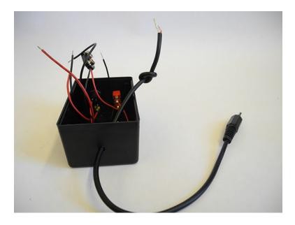
(6) You can now already connect the battery to the 9V clip. Just make sure that the toggle switch is in the OFF position (you can use a multimeter to double check that it is OFF).
