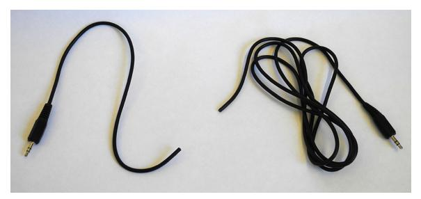
(2) For each of the two cable pieces, take off approx. 0.5in of the cable's insulation, twist together the copper strands:
