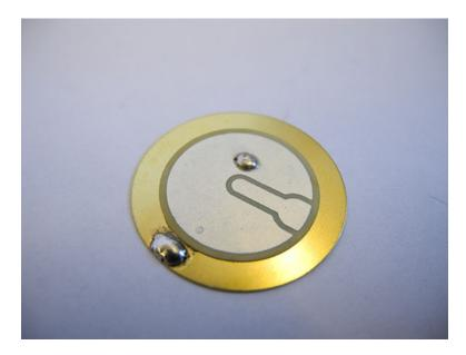
(5) Now solder the longer cable to the piezo disc (reserve the 12 inch shorter cable for later) – the red and white wires go to the white crystal surface in the center, the uninsulated wire goes to the outside rim:
