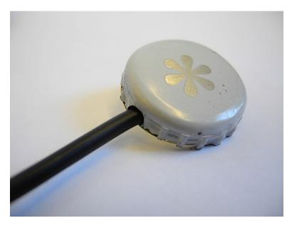
(8) Finally, dip the bottom (piezo side) of the contact microphone into some plastidip and seal around the cable opening on the bottle cap. This makes the microphone water-tight and dampens the microphone's high frequency response a bit.
