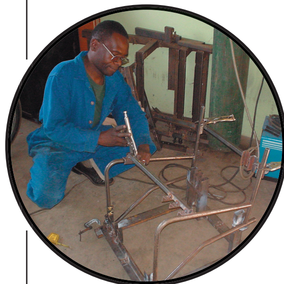
Assembling a Wheel Chair Frame at DISACARE
