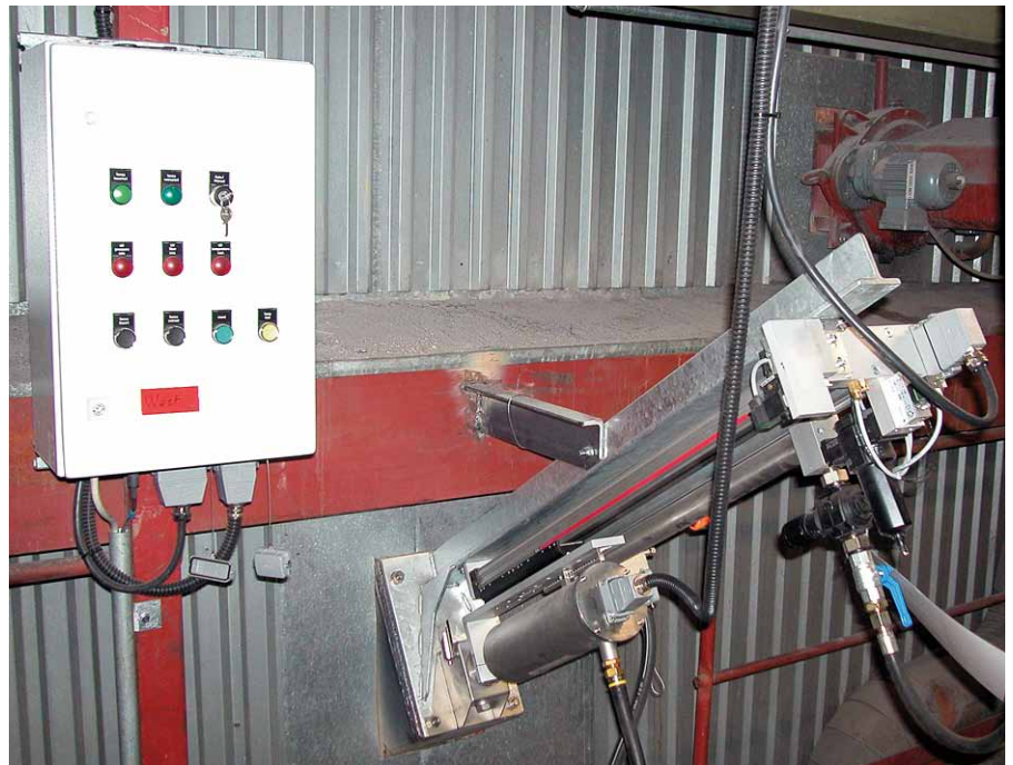
Furnace Camera with Retraction Unit (water-cooled)
