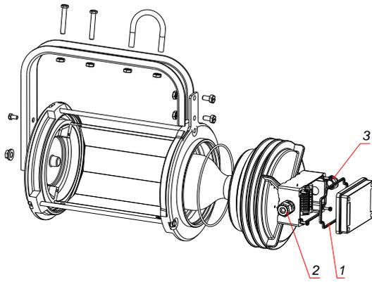
**Floodlight type RLF/... QL** if is not ordered differently, presume floodlight with RLF QL carrier, one Ex e junction box MMK 13 with Ex e connecting terminals, Ex e M25 cable gland, Ex e M25 plug and Philips QL Induction Lighting System, without mounting accessories. Manufacturer will deliver spare part and accessories on buyer request.
