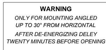
b) Explosion proof floodlight type RLF/... HIT, HST, HME, IQT, IQL with mounting Ex d cable gland are labeled with:
