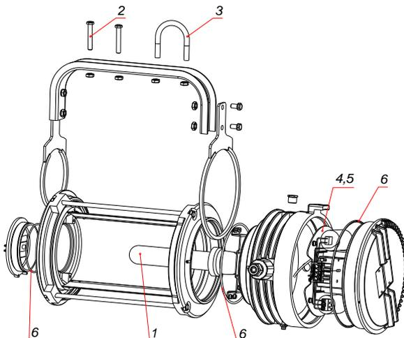
**Floodlight type RLF/ ... HIT, HST, HME, IQT, IQL** If it is not ordered differently, presume floodlight with RLF carrier, one Ex d e adapter ADP 23/1 and two Ex d plugs, without light source and mounting accessories.
