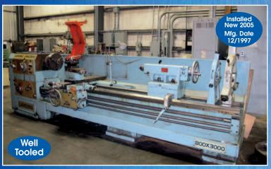
LANSING "GAP TYPE" ENGINE LATHE 31.5" X 118"
