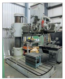
CINCINNATI-BICKFORD # 4E RADIAL DRILL, 6'X 15" CAPACITY
