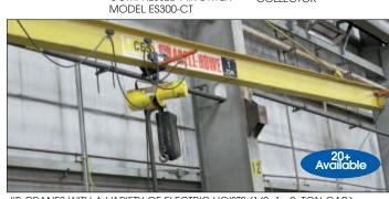
JIB CRANES WITH A VARIETY OF ELECTRIC HOISTS (1/2, 1, 2, TON CAP.)
