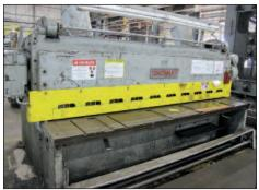
CINCINNATI # 2510 POWER SHEAR 10' X 3/8" CAPACITY
