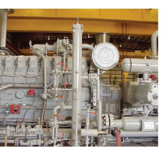
Dresser-Rand's D-VIP compressor uses unique design features of both the HOS and VIP compressors. Like the HOS compressor, the open-frametop construction of the D-VIP compressor ensures rigidity while providing large access areas for maintenance and inspection. Also featured is the throughbolt distance piece design for improved load-carrying capability. The D-VIP compressor also has some unique unloading features that make it one of the most versatile compressors available today.
