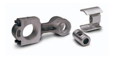
High-strength nodular iron crossheads feature shim-adjustable aluminum shoes at top and bottom. Crosshead pins are full-floating. Integral crosshead guide housings assure positive alignment with the frame.
