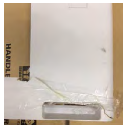
Figure 4 Broken Right Rear Cover
