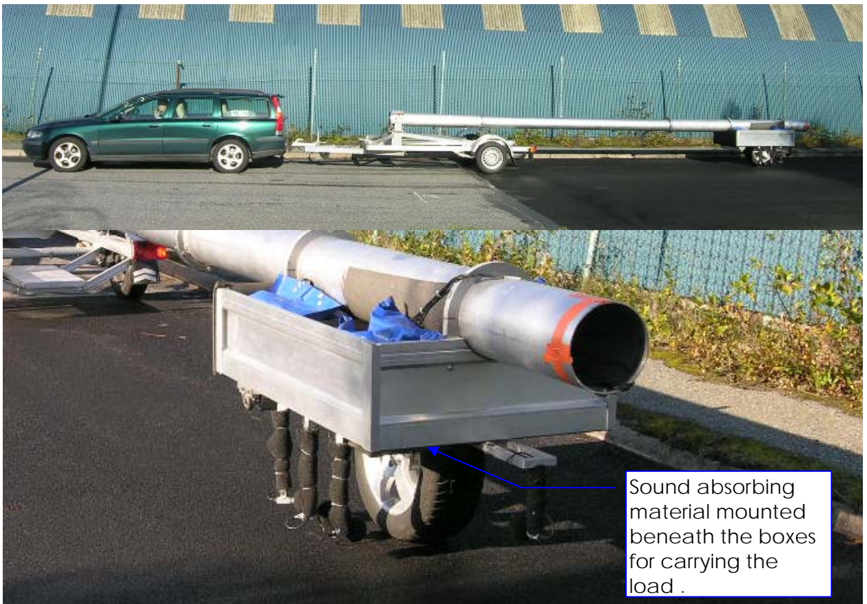
Figure 1. Photo of the single wheel trailer for measurement of tyre/road noise here mounted with a test tyre Goodyear Hydragrip 215/65R15.
