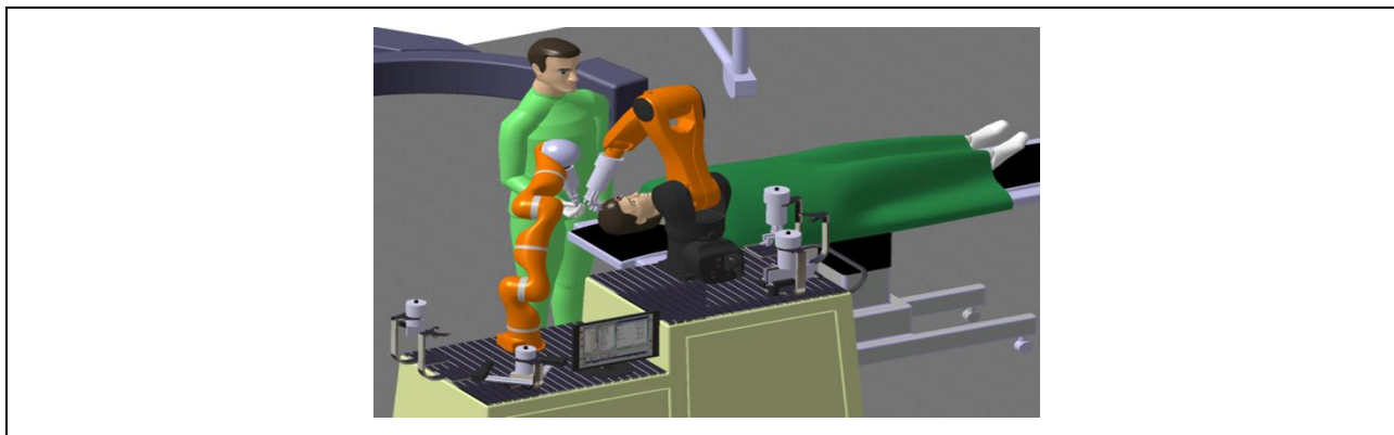
Fig. 15. Location simulation of one variant of the RONNA system in the operating room (Stipančić et al. 2013)
