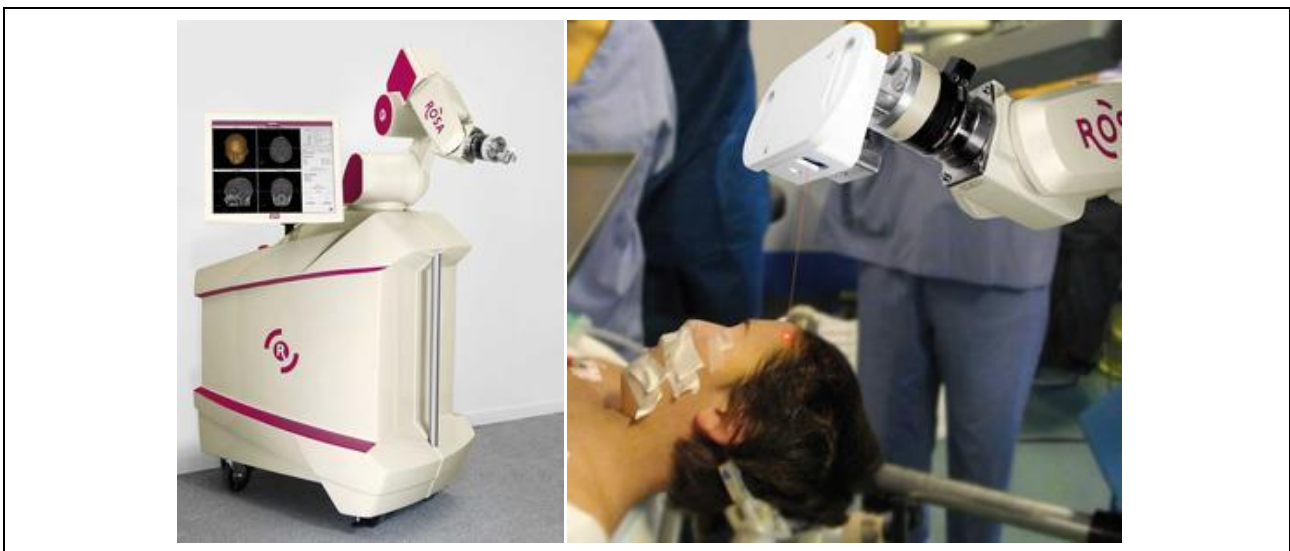
Fig. 6. ROSA neurosurgical robotic system, a) ROSA robot, b) ROSA robot in the operating room
