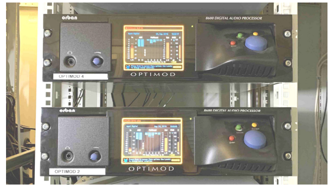
Fig. 11. The broadcast audio processors providing a separate audio processing for analog (FM) and digital (DAB+) platforms, used in the Czech Radio DAB+ network.
