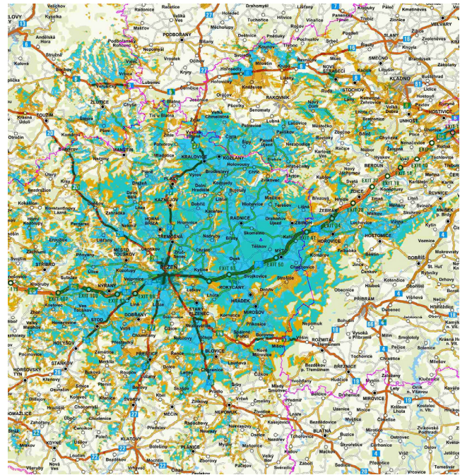
Fig. 8. The numerical modeling of the coverage of the City of Pilsen according to ITU for 66 dB \mu V/m and FEC 2A - without an additional city transmitter.
