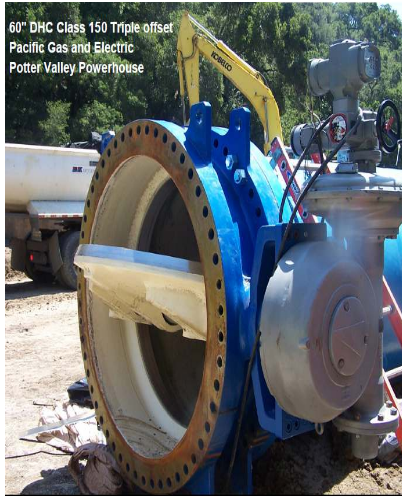
Pacific Gas and Electric Potter Valley Powerhouse Class 150 60" Triple offset Butterfly
