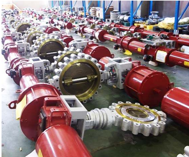
CONTROL BUTTERFLY VALVE ALGERIA SKIDDA PJT PNEUMATIC ACTUATOR
