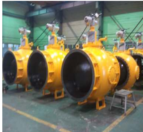
WATER SEAL VALVE 1500A APPLICATION : COG/BFG/LDG
