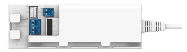
Aux1 to Aux1C and Aux2 to Aux2C Connections are Dry contacts (contacts are rated for Max 24VAC)
