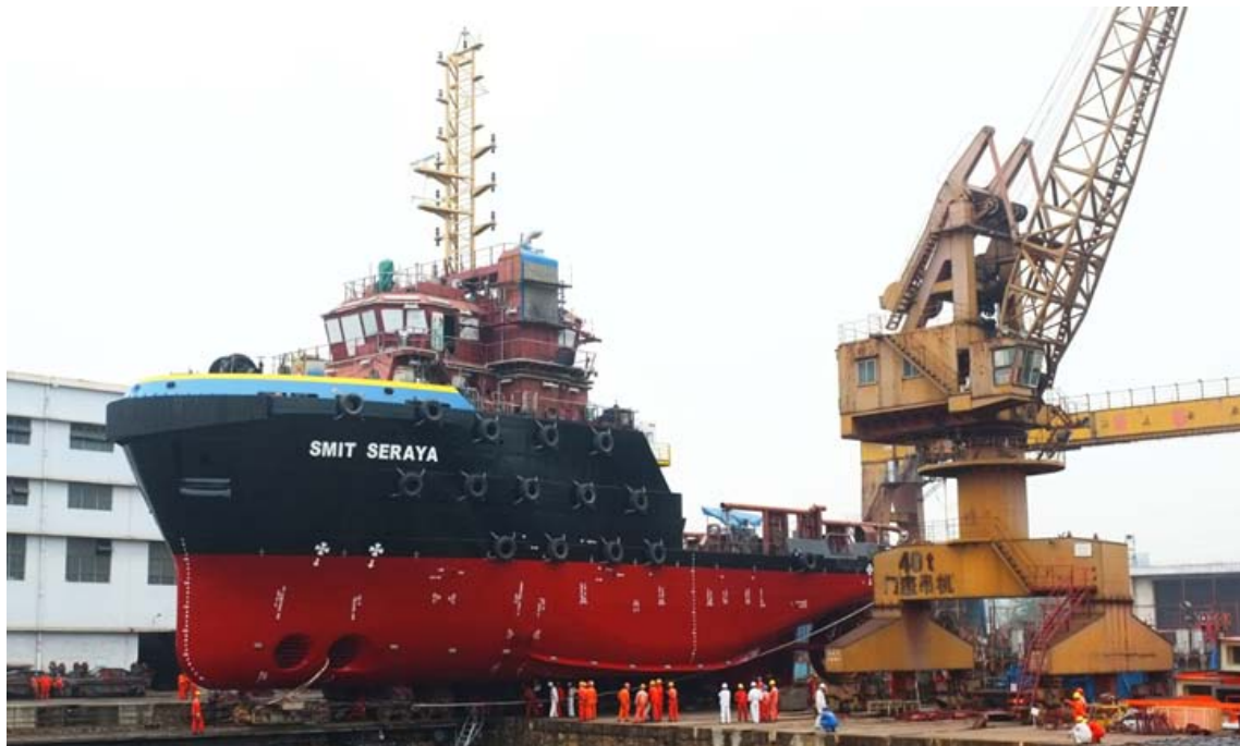
The 7300 hp ( 95 ton BP) SMIT SERAYA under construction at the Lingsian Yard in Wuzhou China Photo : Capt John Bruinsma ©
