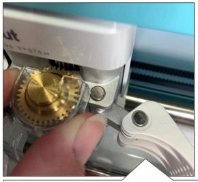
Cricut will prompt you when it's ready to use the tip. Open clamp 'B' and insert the housing so that the gears meet and then reclose the clamp.
