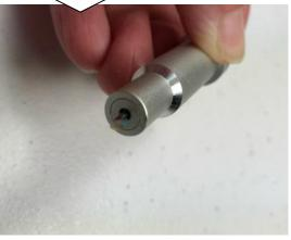
To get more use out of a blade depress the plunger and stab it into a ball of tinfoil several times to clean and re-sharpen. Please be careful that you don't stab yourself
