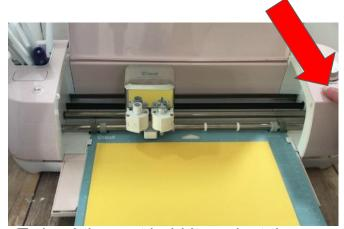
To load the mat hold it against the roller bars and press the load/unload button. When your cut is complete press the load/unload button again to release the mat.
