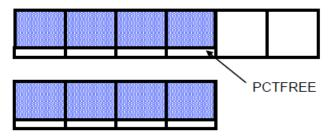
Backward scan starts at end, fills holes earlier in table identified by simultaneous forward scan. Can be <u>significantly</u> faster than the reclustering option, as it typically requires far fewer row moves.
