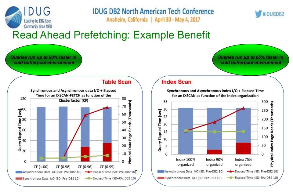
As of V 10.1, DB2 performs read ahead and sequential prefetching automatically, as appropriate
