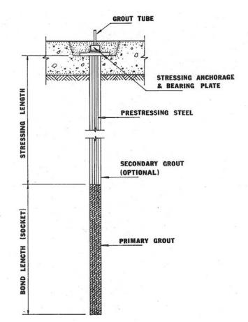
**Figure 1.** Rock Anchor Components (PCI, 1974). (Note the lack of protection to the steel other than cement grout.)
