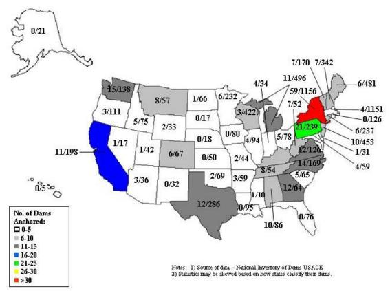
Figure 7. Geographic distribution of U.S. dams which have been anchored.
