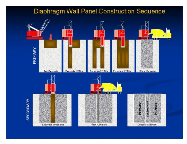
Figure 9. Diaphragm wall panel construction sequence.
