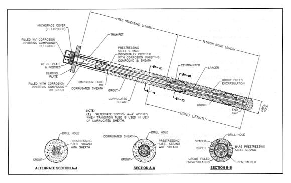
Figure 2. Class I Protection – Encapsulated Strand Anchor (PTI, 2004).
