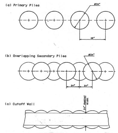
Figure 10. Construction sequence for a secant cut-off wall (Bruce and Dugnani, 1995).
