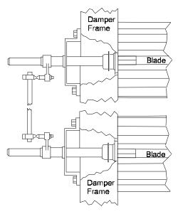
DMPR-KC101 vertically couples two panels for an external drive. It is used with either both panels open, or one panel open and the other panel closed.
