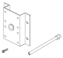
This kit includes a blade pin extension and a bracket with a bearing that attaches to the end channel to provide additional support of the blade pin extension. Use this kit for support when the universal mounting bracket is not used.
