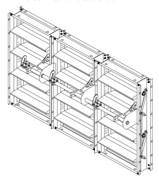
DMPR-KC206 couples three panels to the same actuator. The actuator should be situated near the center of the jackshaft for best results. The jackshaft length is 10 feet.
