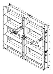
DMPR-KC205 provides an extended drive location, or couples two panels to the same actuator. The actuator should be situated near the center of the jackshaft for best results. The jackshaft length is 5 feet.
