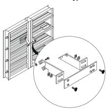
DMPR-KC150 horizontally couples one normally open and one normally closed panel, joined side by side in a face/bypass configuration. This application requires one panel to be ordered with left side linkage. One kit is required for every 24 inches of panel height.
