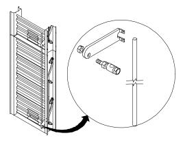
DMPR-KC100 provides all components necessary to drive vertically coupled panels. It uses a 48-inch-long, 5/16 inch diameter linkage rod. Face/Bypass application requires one panel to be ordered with left side linkage.
