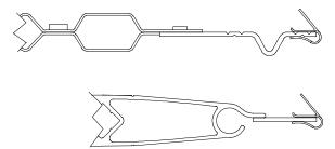
DMPR-RC054 is used with double-piece and airfoil blades with extensions for top and bottom blades.
