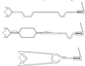
DMPR-RC006 is used with double-piece and airfoil blades, top and bottom with extensions, and all 16-gauge blades manufactured after date code 0696, in parallel and opposed operation.
