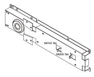
DMPR-KC255 is used to mount an M9000 series actuator to a CD-1300 damper inside the airstream.
