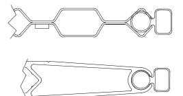
DMPR-RC002 and DMPR-RC051 are used with double-piece and airfoil blades in opposed operation.
