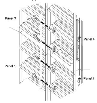
This kit includes one 21-inch-long bar to be installed at the point where four panels join.
