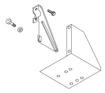
DMPR-KS101 provides the parts required to convert a smoke damper with an external factory-installed electric actuator to an internally mounted actuator on the right side.
