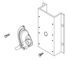
DMPR-KC250 provides for manual positioning and locking.
