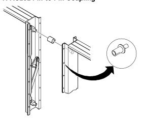
DMPR-KC202 horizontally couples panels pin-to-pin. Order one kit per 48 inches of panel height. Install a coupler on every pin.
