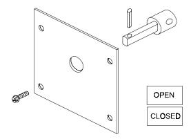
DMPR-KF001 provides a visual indication of the FD-1300 fire damper blade position.
