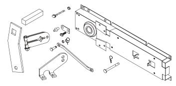
DMPR-KC254 kit is used to mount an M9108, M9116, M9124, or M9216 actuator to a Johnson Controls damper inside the airstream.
