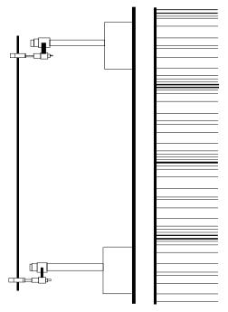
DMPR-KC102 is a 48-inch-long, 5/16 inch diameter connecting rod for linkage kits.
