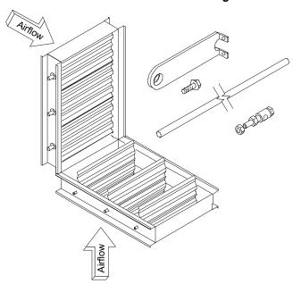
DMPR-KC152 couples two panels joined at a 90° angle. Panels should be normally open/normally closed, and this kit should be used on panels with three or more blades. Requires one panel to be ordered with left side linkage.
