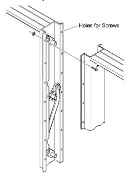
DMPR-KC201 is used to secure two or more panels together. Order one kit for each 48 inches of panel height.
