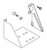
DMPR-KS102 provides the parts required to convert a smoke damper with an external factory-installed electric actuator to an internally mounted actuator on the left side.
