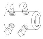
DMPR-KC006 is a coupler used to join two blade pin extensions to accommodate separations between two panels.
