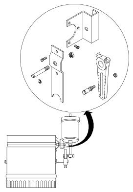
DMPR-KR001 adapts a D-3062 actuator for installation on a 9 to 16 inch (229 to 406 mm) RD-2000 round damper.
