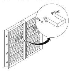
DMPR-KC151 horizontally couples two panels with the blades operating in the same direction. One kit is required for every 24 inches of panel height.
