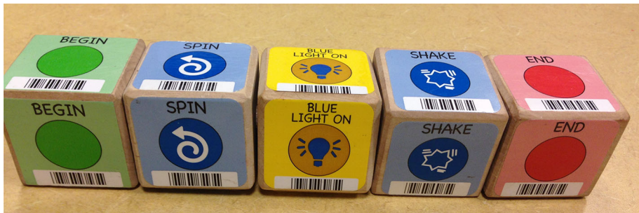
Fig. 2 Sample KIBO program. This program tells the robot to spin, turn a blue light on, and shake
